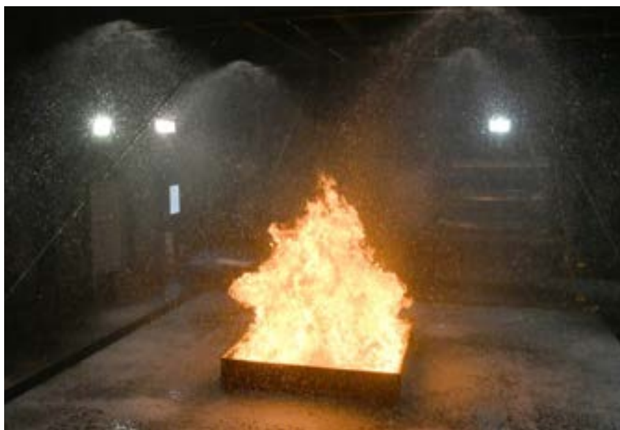
Testing of ANSUL NFF-331 AR-SFFF at 3% concentration on heptane fuel fire per UL 162 test protocol.
