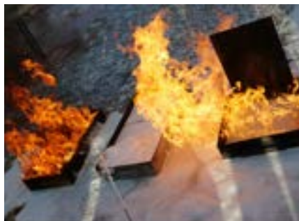
Figure 5: influence of application technique: application of the same foam quality for the same application time on three different fuels the used foam agent is suitable for
