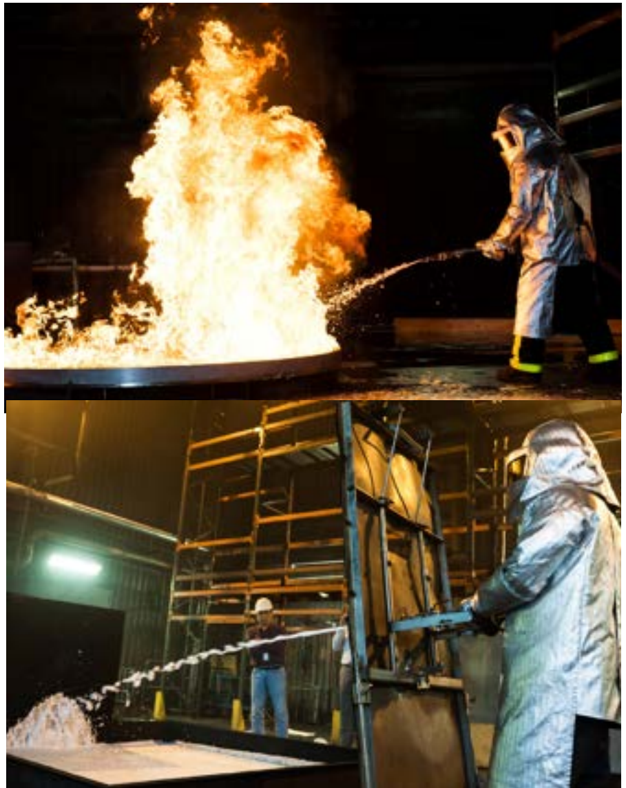
Figure 2: Testing with forceful (type III) and gentle (type II) application methods
