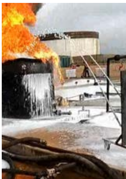
Monitor application to crude – with some slopover
