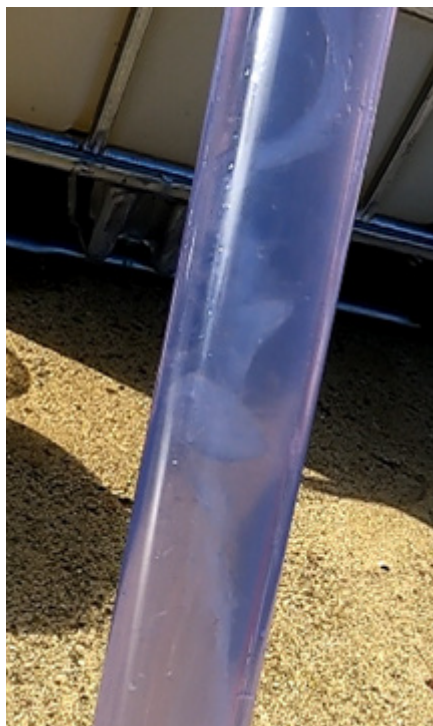
A “string” of unmixed foam concentrate in the water stream observed under some conditions during LASTFIRE research
