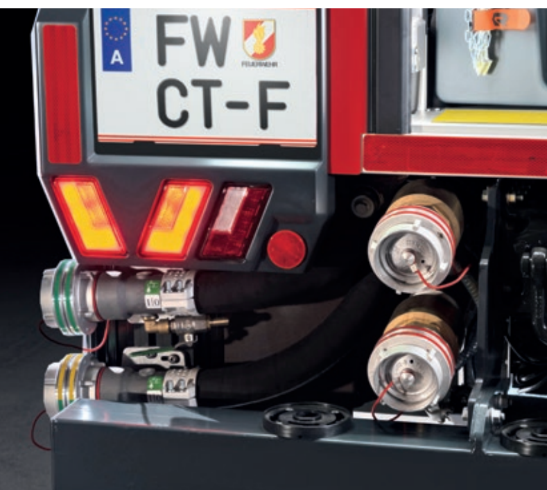
Central water supply and external side pressure outlets.
