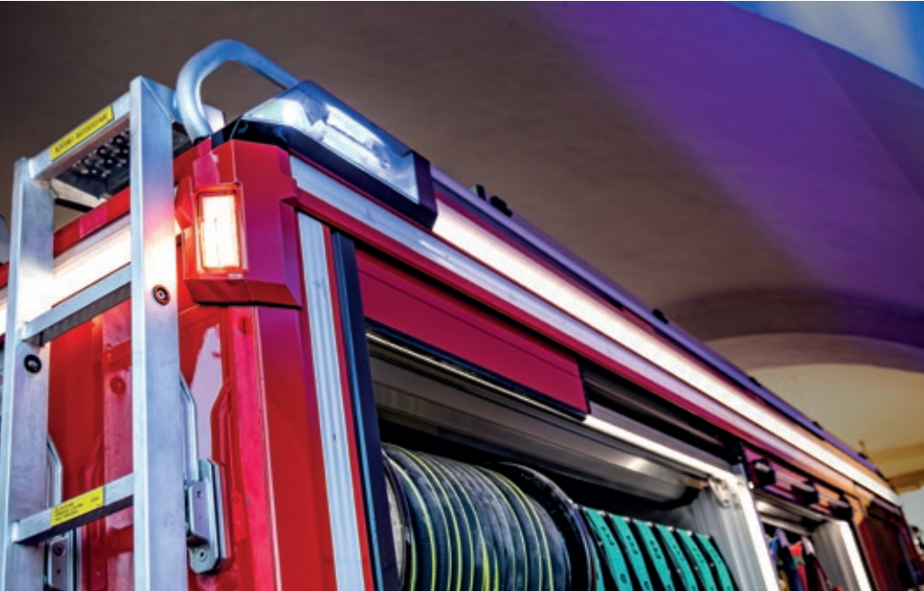
High-performance LED strips in the roof gallery.
