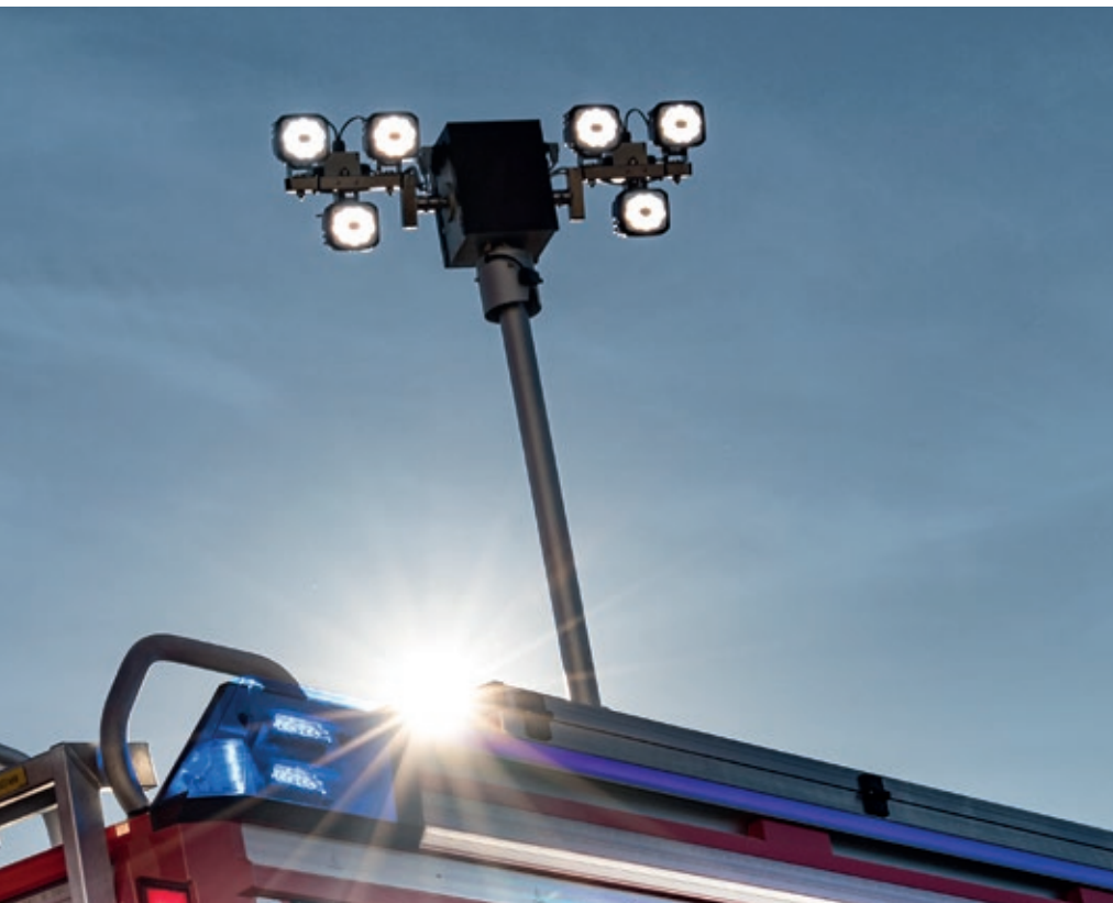
Pneumatically extendable light mast.
