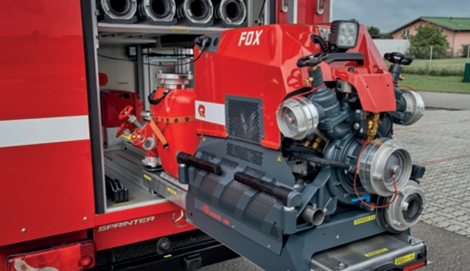
FOX on pull out platform, installed at the rear.
