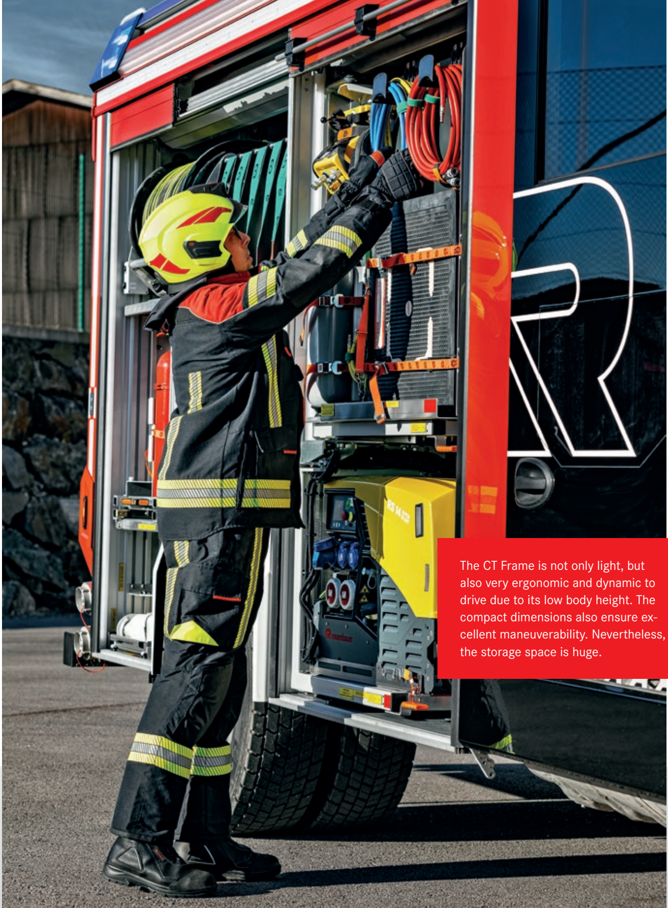
Full-height roller shutters all the way down for convenient removal of equipment.
