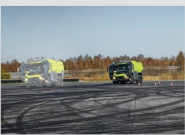
Driving through corners at high speed without / with RSC
